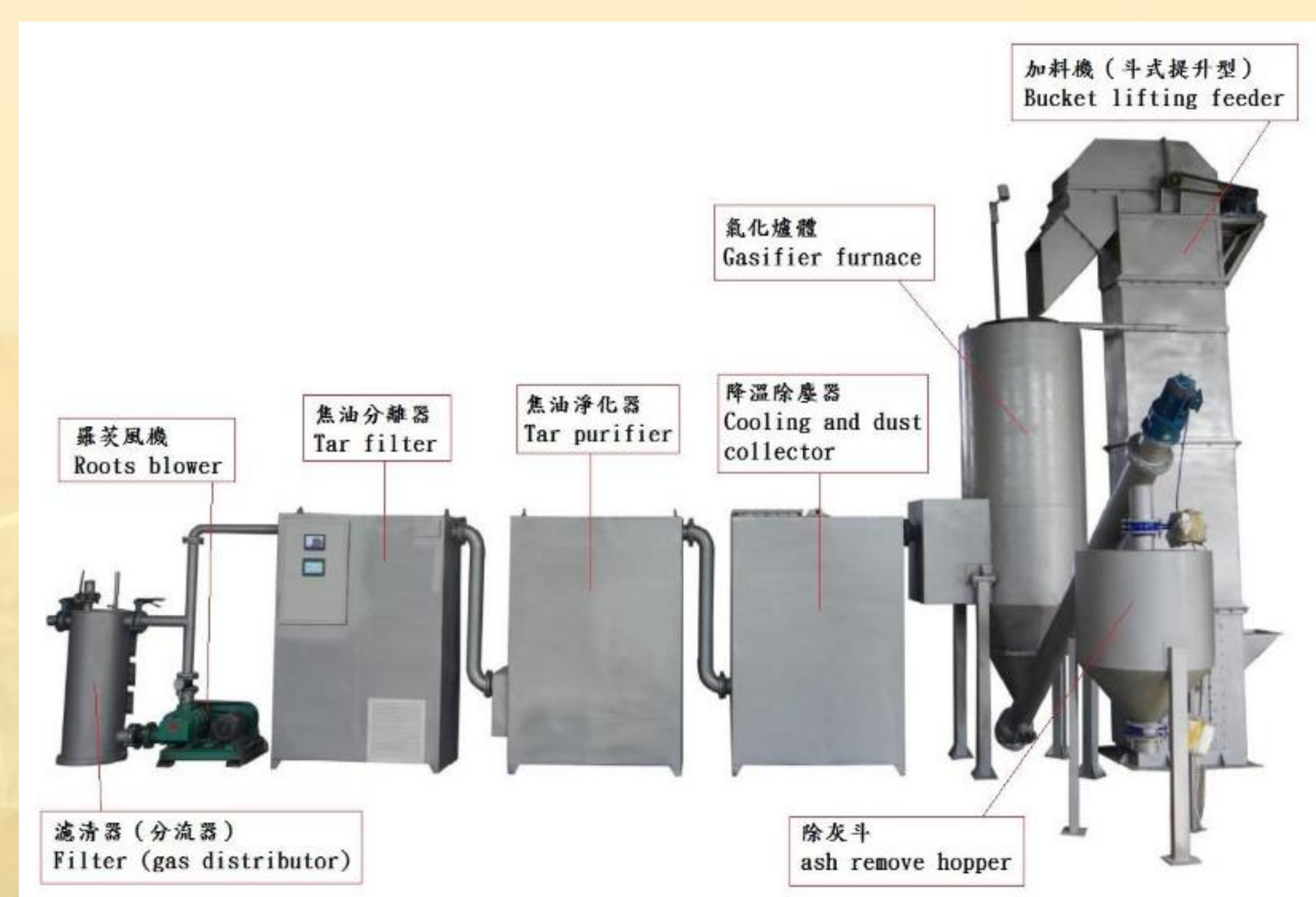
Figure 2. 100KW biomass gas power generation equipment
